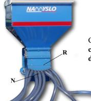
Connect the **seed tubes** (**N**) with one end to **the plates** (**P**) with special **clamps** (**O**), and the other end to the correct ends of the **grain distributor** (**R**) (push the seed tubes over the ends of the distributor).
