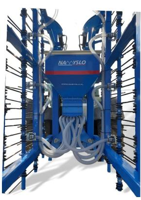
The SPREAD P seeder has been designed in such a way that the machines from the NAMYSLO Damian Namysło offer, on which it can be attached, and whose working width exceeds 3 meters, folded into the transport position without collisions. The tracking wheels of the catch crop seeder mounted on such aggregates cannot be folded for transport,
