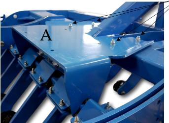
Using the attached mounting plate - adapter (A), you can mount the catch crops seeder on various types of machines.
