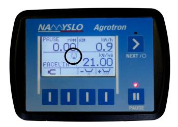
Controlling the filling level of the tank grain during work, without leaving the tractor, the indicator on the controller allows.
